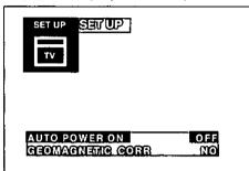
NOTE: Setting the Auto Power On feature will cancel the time and timer control setting. Also, the TV Mode Main Menu Icon for the Control will be replaced with an
